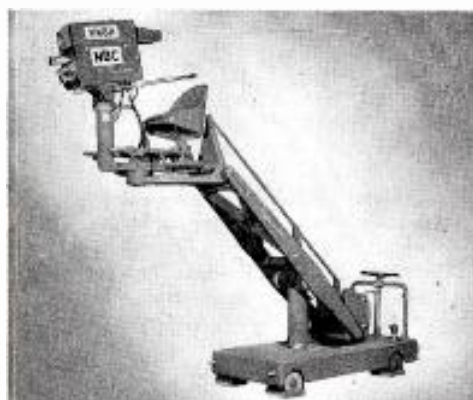
HOUSTON-FEARLESS TC-1 CRANE raises camera to extremely high and low positions. Permits "fluid motion" shots. Foot-operated panning.
